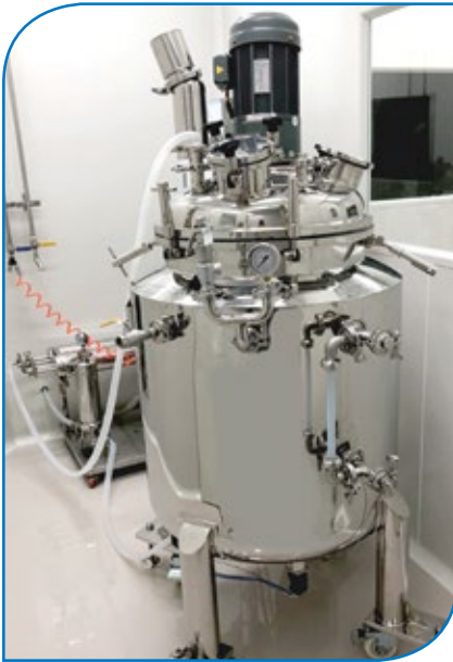
AUTOMATICAL DISPENSION TANK OF INJECTION SUSPENSION
